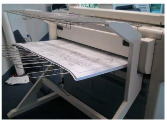
NOTE: The centre guides are used to prevent the prints from rolling up as they exit the printer. This can occur in high humidity environments and or near the end of a paper roll where the curl is more progressive. Reinstall the centre guides if necessary.
